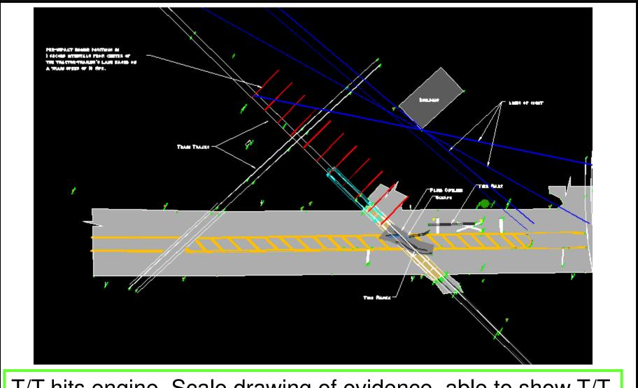
T/T hits engine. Scale drawing of evidence, able to show T/T had ample time to perceive/react and stop.
